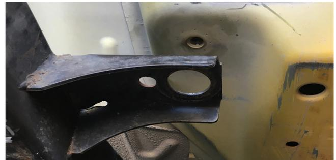
**STEP 3.** Using either a plasma cutter or a grinder with a cut off wheel, remove the factory side body mounts. Grind the frame smooth around the body mounts until it is bright shiny metal. This will ensure a good surface to weld to.
