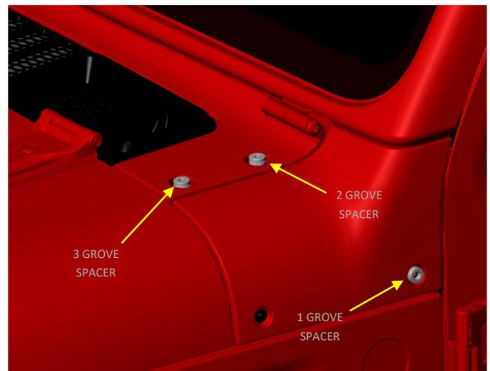
STEP 5. Install the driver side brackets. Use two 50mm long bolts in the top of the cowl, and one 30mm long bolt in the side of the cowl. Tighten these bolts down.
