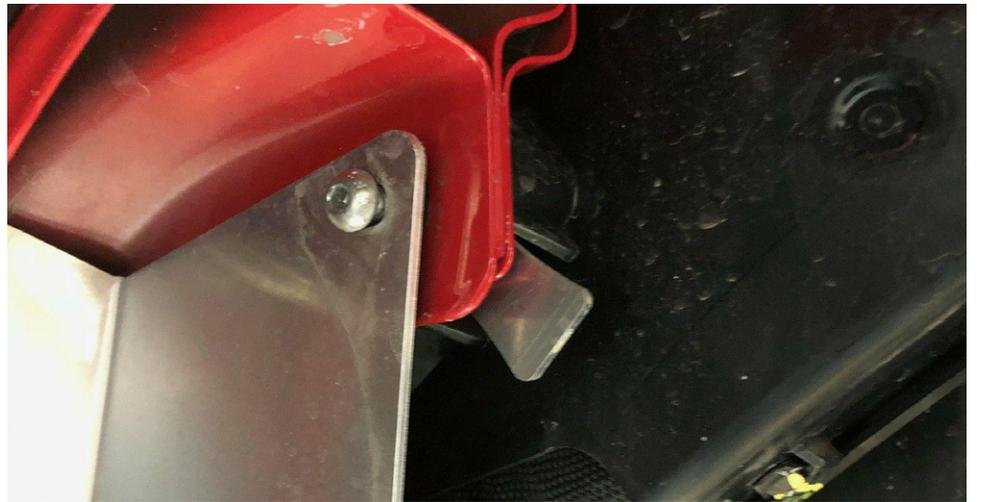
**STEP 7.** If your installing the trim to fit fenders ensure there is proper clearance around all aftermarket suspension brackets. Prior to final install we recommend that the inner fenders be painted, or powdercoated. Some also choose to wrap them in vinyl. The fenders are raw aluminum and will corrode over time. Perform the final install and use blue thread locker on all the fasteners to ensure they do not vibrate loose over time.
