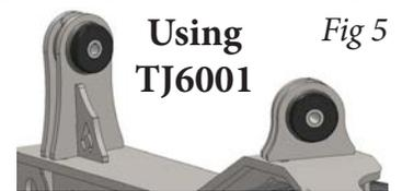
**STEP 8.** Once mockup is completed and results are satisfactory, grind off the tack weld on piece 1 (truss top) and remove. Weld the inside of the truss gussets using the techniques in **GENERAL WELDING INSTRUCTIONS** above. Replace piece 1 on the truss and begin final welding of all pieces. Remember to take your time and spread out your welds. It is not necessary for every seam to be completely welded. Let cool slowly as described above.
