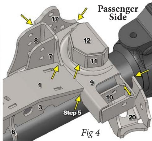
**STEP 7.** Installation of the UCA brackets will vary depending on the style you choose. For Bushings and Johnny Joints, the parts labeled TJ6001 will jig into the predetermined slots on part 1 (truss top). Follow the diagram for placement. Center the tube sleeves between the two tabs for welding. For the 3-link bracket, place on top of part 1 (truss top) centering the bracket on the slots cut out for the TJ6001. Mock up with your existing upper link prior to final welding.
