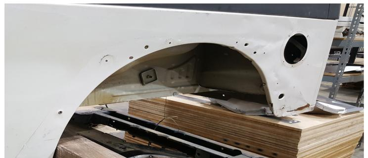
**STEP 3.** Next prepare the surface by wiping all the dirt off to prevent paint damage during install. Once the jeep is dry and clean apply painters tape on the jeep around the perimeter of where the corner armor is going to sit. This will prevent the paint from getting scratched.
