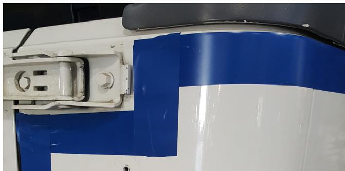
**STEP 4.** With assistance place the corner armor on the vehicle and clamp into place. Once its clamped to the jeep you can fine tune the alignment with a rubber mallet. Ensure that mounting holes line up for the gas tank filler, tail lights, and license plate. Inconsistency between jeeps is not uncommon.
