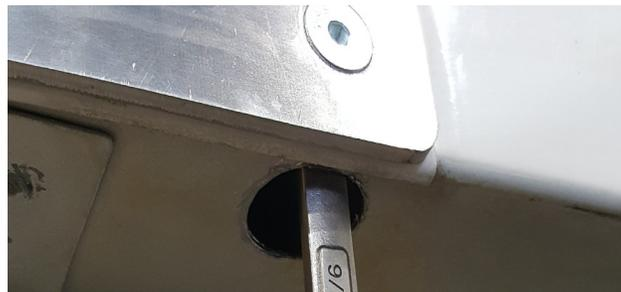
**STEP 7.** Once all the bolts have been installed you can either install the factory tail lights or use a hole saw to cut out for a round tail light. Also re-install the fuel filler, license plate mount and plastic caps on the passenger side hinges for a clean finished look. Once you have verified everything fits you can opt to remove the armor and have it painted or powder coated.
